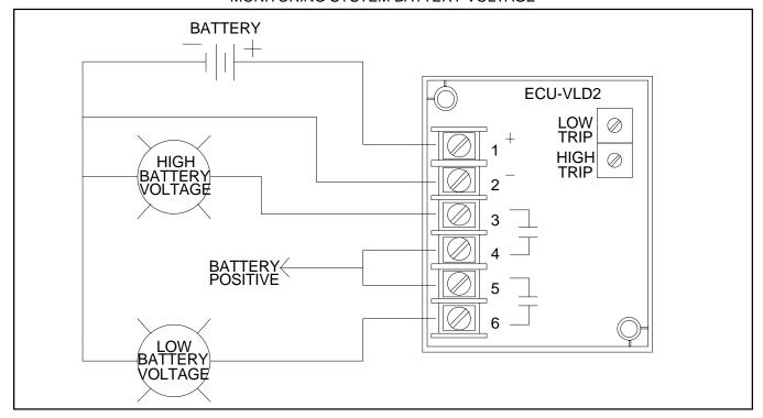
The above example is the most popular application of the voltage detector module. The lamps will track the voltage condition as programmed by the trip adjustments.
