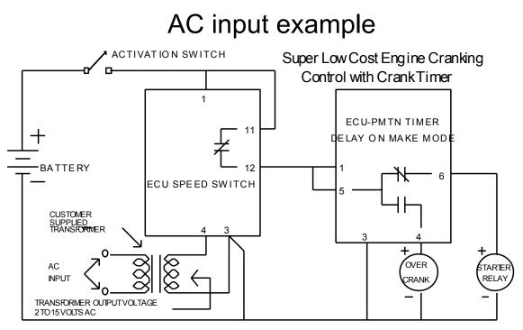
SS21 Speed switch AC transformer operation
