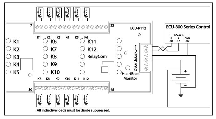
The above connection diagram is a typical multi input system using RS485 Modbus . As long as the unit is operating Heart-beat monitor led will blink. Final units in the 485 chain must be terminated by 120ohm resistor. Use twisted pair shielded wire and you can achieve lengths as far as 4000 feet.
