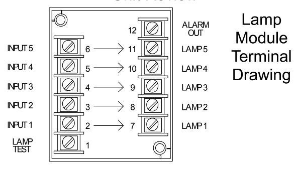
The LTO2 AND LTO4 are highly flexible design components. It was originally developed for annunciation. It is still used for this and also for system fault isolation and lamp control. The LTO2 is shown for example but the LTO4 is identical in operation except for having for more lamp circuits.
