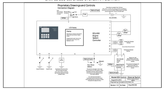
In the above application, the ECU-GAUGE can be seen attached to an ECU-800 series controller, via a  $120\Omega$  terminated shielded twisted pair. This will be used for MODBUS signaling between the ECU-800 and the ECU-GAUGE. It is notable that multiple ECU-GAUGE modules can be addressed by a single ECU-800 series controller.
